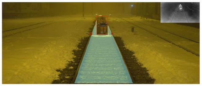
Human & braking shoes detection at night and in harsh weather conditions
