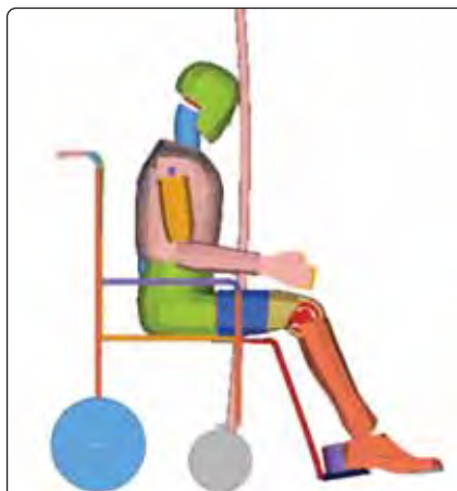
Figure 4: Wheelchair occupant secondary collision with a grab pole
