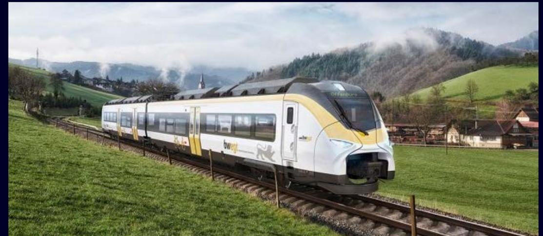
The Mireo Plus B battery hybrid train features operation that is extremely cost- and energy-efficient as well as locally emission-free. This makes it ideal for modern, European regional transport as a smart alternative to conventional diesel multiple units, especially on non-electrified or only partially electrified lines.
